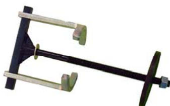
KA-5003 Automatic Transmission Clutch Spring Compressor
