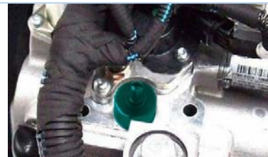
Install the tool to lock the selection lever inside the actuation hydraulic unit.
