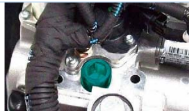
Undo the protection plug for the hydraulic unit selection lever locking tool.
