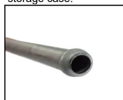
Completed metric bubble flare
