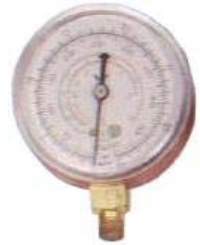
KA-7405H Gauge pc cover high side 0 to 500 psi 1/8" NPT connection 2-3/4" dia scale for R134a & R12
