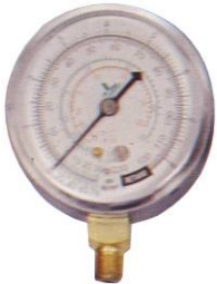
KA-7405L Gauge pc cover low side 30 to 250 psi (vacuum) 1/8" NPT connection 2-3/4" dia scale for R134a & R12
