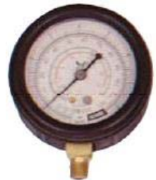
KA-7406L Gauge pc cover low side 30 to 250 psi (vacuum) 1/8" NPT connection 2-3/4" dia scale for R134a & R12
