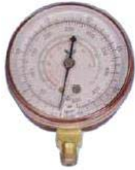
KA-7404H Gauge pc cover high side 0 to 500 psi 1/8" NPT connection 2-3/4" dia, red color scale for R134a & R12
