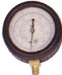
KA-7406H Gauge pc cover high side 0 to 500 psi 1/8" NPT connection 2-3/4" dia scale for R134a & R12
