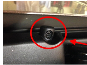
Four slotted good for adjust windsreen nozzle
