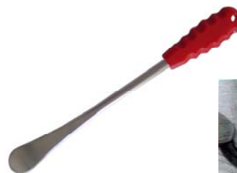
KA-7022 Tire Lever Suitable for passenger cars, motorcycle and industrial tyres. Made with high quality drop forged and tempered alloy steel. Length: 11"(280mm) Width:1"(25mm)
