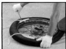
KA-7023 Rim Protector Convenient tool while changing the tire with the weight
