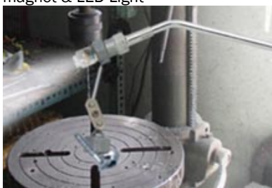
Attract small parts in dark place by magnet & LED Light
