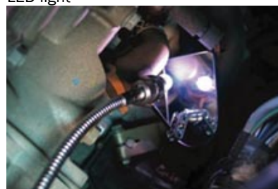
Inspect parts in dark place by mirror & LED light
