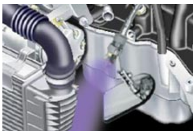
Detect radiator leak with UV light
