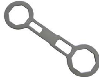
Fork Cap Wrench For removing the fork caps on late-model RMs & CRs Can be used for removal of a compression stack on late-model RMs KA-2950 46~50mm KA-2951 49~50mm
