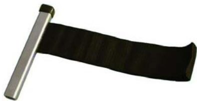
KA-2013 Nylon Strap Oil Filter Wrench Use wrench on oil filters up to a 6" (152mm) capacity. Strong nylon belt will not slip. Use with 1/2" square drive tools. 2" Wide
