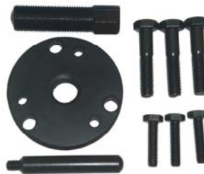
KA-4186 Flywheel puller ■ Puller kit designed to pull magneto flywheel or starter gear. ■ Includes three 6 x 25mm and three 8 x 40mm bolts. ■ Applications: Kawasaki Jet Ski 300/440/550, Yamada WR250F 01-02 and WR400F flywheel.
