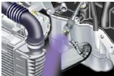
Detect radiator leak with UV light
