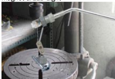
Attract small parts in dark place by magnet & LED Light
