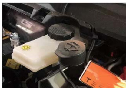
Fig. 2 Locate the master cylinder reservoir
