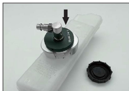
Fig. 4 Insert the adapter into the filler neck
