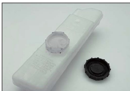
Fig. 3 Remove the reservoir cap
