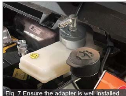
Fig. 7 Ensure the adapter is well installed
