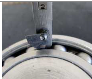
Step1: Select correct jaws and shim according to the bearing gap
