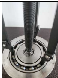
Step 3: Ensure the jaws are installed firmly
