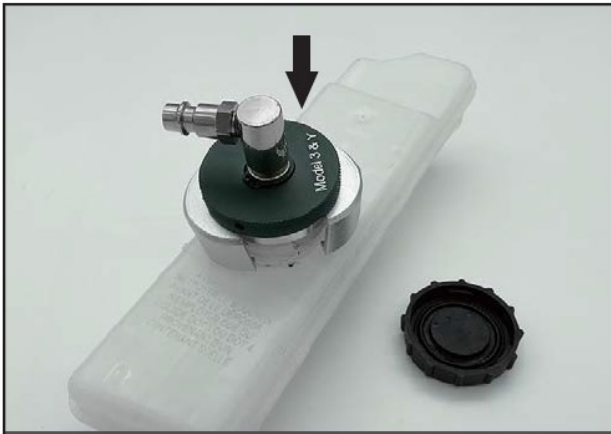
Fig. 4 Insert the adapter into the filler neck
