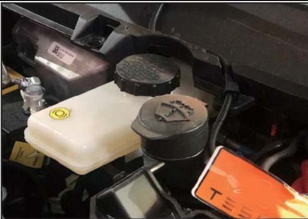
Fig. 2 Locate the master cylinder reservoir
