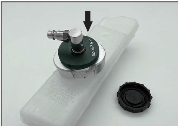
Fig. 4 Insert the adapter into the filler neck
