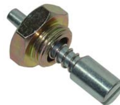
KA-2877 Injection Pump Lock Pin-Late Model ■ Locks diesel pump cam to maintain timing during pump installation ■ Mercedes Benz: 601, 602, 603, 604, 605, 606, and 617.
