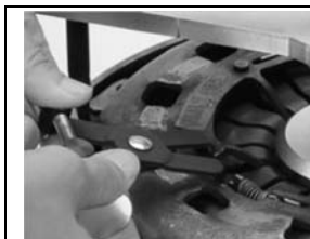
If the old clutch cover is to be re-used, it must first be reset. The adjuster ring can be turned back with clutch resetting tool.
