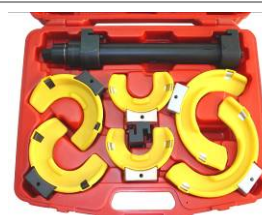
KA-7309KA-AIR The yellow plastic covers could protect the surface of shock absorber.
