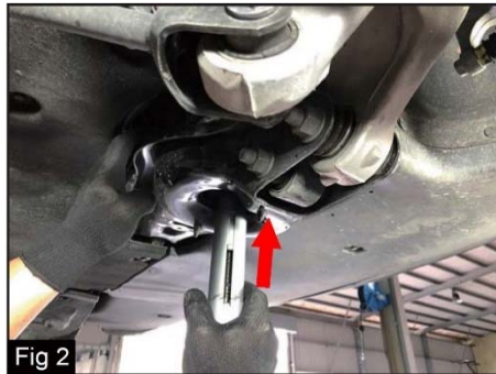
Insert the main tool body into the spring.
