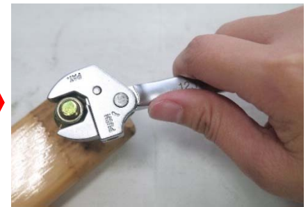
Drive the clamp to tight and release the nut.
