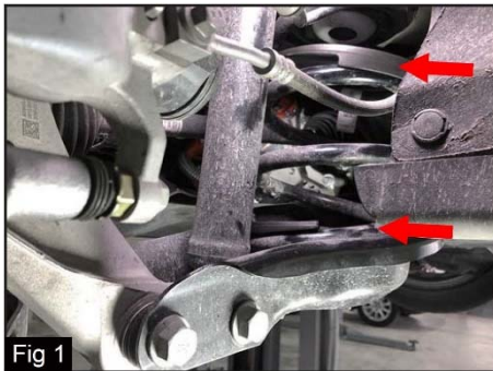
Place upper and lower discs on spring.
