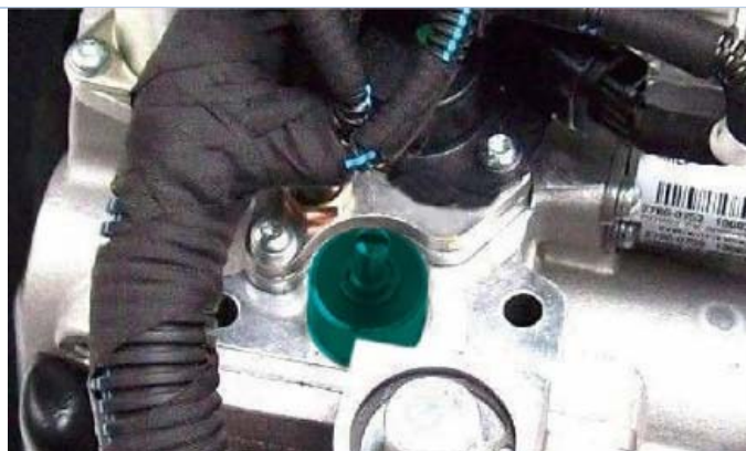
Install the tool to lock the selection lever inside the actuation hydraulic unit.
