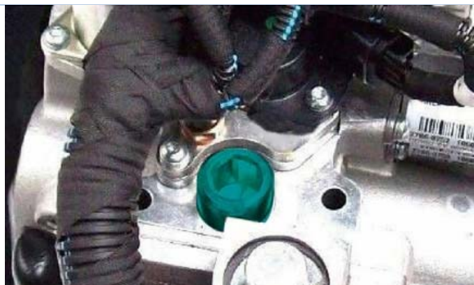
Undo the protection plug for the hydraulic unit selection lever locking tool.
