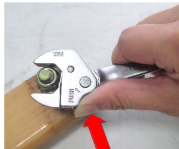
Push the jaw to open the calmp onto the nut.
