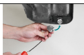
Place the tool on plug so that the tool locks on the plug hex
