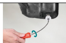
Rotate handle to remove plug
