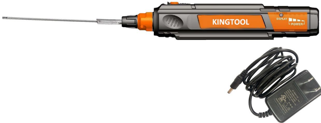
KA-5888C10 70W Styrofoam Cutter , Max Temp 450°C (842°F)
